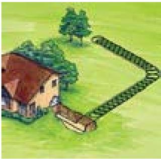
**Horizontal Slinky Loops:** Another type of horizontal loop is called the Slinky. In this installation, a trench is dug with a backhoe several feet deep, and about 3 feet wide. The coils are "laid off" and spaced evenly throughout the length of the trench. (Think of a flattened, stretched out slinky toy.) Slinkys can be designed as "compact" or "extended". Trench lengths are typically 100 to 150 feet long.
